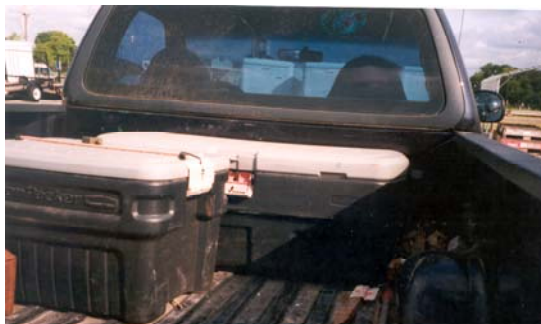
No. 10 Hazardous materials in unsecured storage inside plastic boxes in the bed of a pickup truck.
