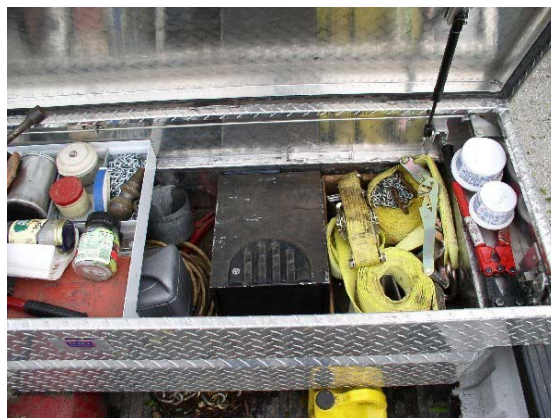
No. 11 Example of proper storage for hazardous materials stored on the bed of a pickup truck.
